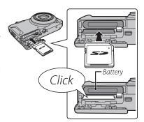
• SD/SDHC/SDXC memory cards can be locked, making it impossible to format the card or to record or delete images. Before inserting an SD/SDHC/SDXC memory card, slide the write-protect switch to the unlocked position.
